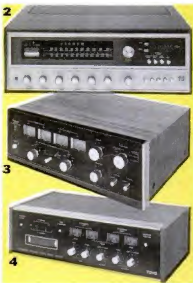
A SEEMING IMPOSSIBILITY —playing four channels from a single record groove—is accomplished by this Japanese Victor decoder to be marketed soon. It will work with any high-frequency phono pickup
